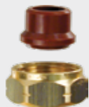
SVC compression adapter - Only for type L copper, type K copper, type M copper - Brass - SVC - Allows compression copper connection with SVC manifold without soldering Components Brass nut, plastic insert Model 9438.5SV
