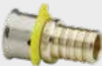
Viega PureFlow Press adapter Zero Lead - Bronze - Press connection, polybutylene (PB) connection - Does not include crimp ring Model 2813.2ZL
