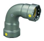
MegaPressG for Marine is a carbon steel, cold press system designed for use in a variety of marine and offshore applications. It requires no threading, welding, or grooving and poses no fire hazard. The press fittings are installed with a hand-held
