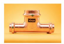
Viega ProPress may only be pressed onto copper tube in accordance with ASTM B88 or B75. When pressing onto B88 copper tube, types K, L, and M may be used. Tempers O60 and O50.
